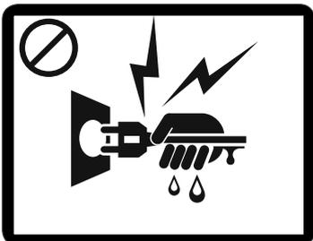
Do not remove the plug by pulling on the cord; handle it by the plug end only; do not handle the plug with wet hands. This could result in electric shock or fire.
